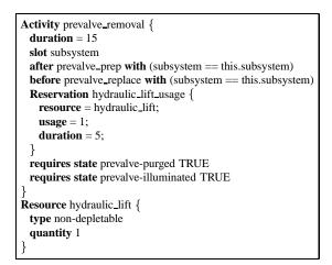
Figure 1: Sample of ASPEN modeling language (part of the Reusable Launch Vehicle maintenance model). This describes an activity for removing the prevalve of an engine subsystem.
